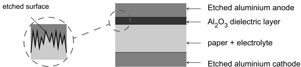
Figure 3.13 Electrolytic capacitor construction
